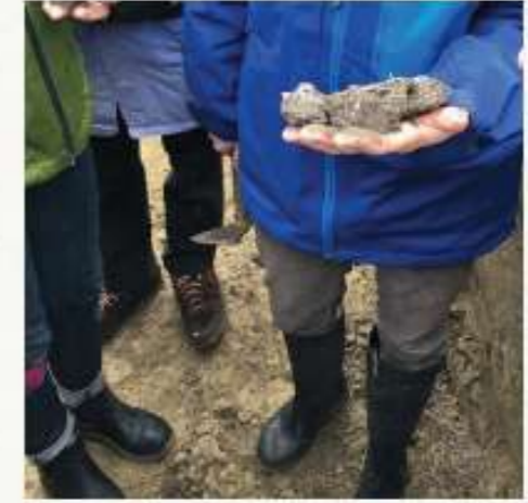
Identifying soil constituents: silt, sand, and clay by touch
